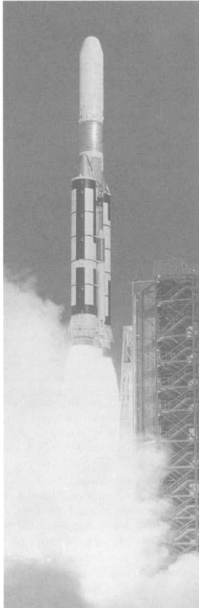
FIGURE 1-12. Titan III launch vehicle shortly after lift-off, with bright radiant exhaust gas. Two solid propellant rocket motors, each providing about 2.4 million pounds of thrust, boost the first stage, which also gets a sustained thrust of 470,000 pounds from two liquid rocket engines. The second stage has 100,000 pounds of thrust from a single liquid rocket engine, and one version of the third stage has two liquid rocket engines, each at 16,000 pounds of thrust.
